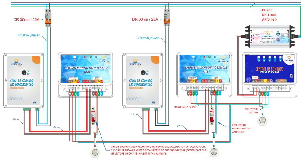
NOTE: NECESSARY TO INSTALL A CIRCUIT BREAKER ON THE POSITIVE WIRE OF THE CIRCUIT THAT FEEDS THE REFLECTORS, FOR TOTAL GUARANTEE THAT THERE WILL BE NO DAMAGE TO THE FACILITIES AND EQUIPMENT. DISRUPTIONS MUST BE DIMENSIONED ACCORDING TO THE CIRCUIT LOAD AND THE CURRENT LIMIT OF THE ELECTRICAL CABLE.
