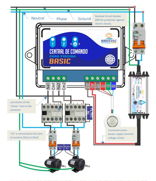
WE ADVISE INSTALLATION OF THIS EQUIPMENT IN AN OPEN AND VENTILATED PLACE TO AVOID PROBLEMS LIKE MOISTURE AND OXIDATION WHICH NORMALLY OCCUR IN ENGINE ROOMS.
